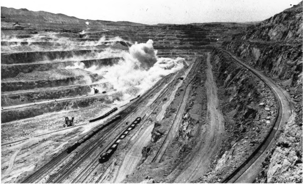
78 One section of huge open cast copper mine at Chuquicamata, Chile, showing the series of terraces cut out by power shovels which form working levels for further excavation
